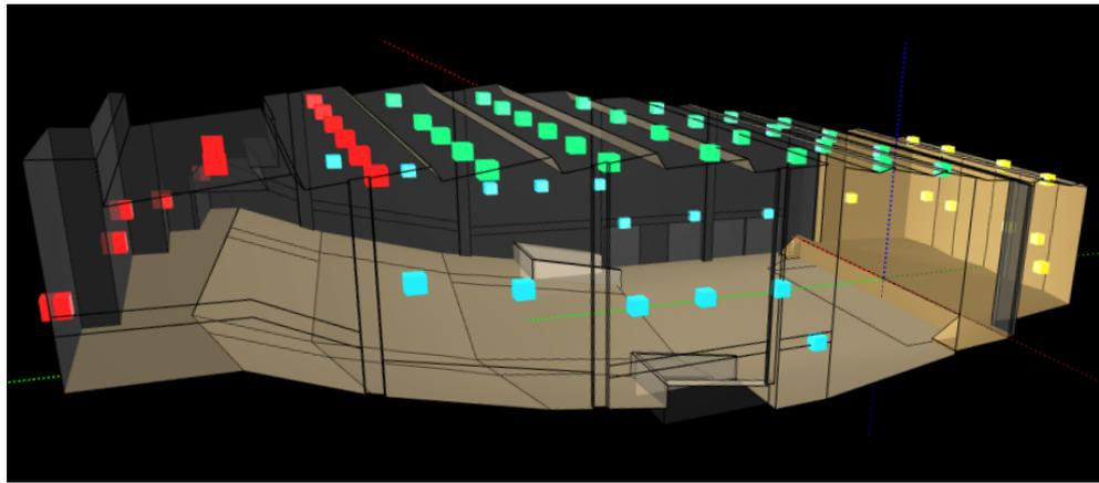
**Figure 4.12.** 3D-Model of the Konzerthaus with loudspeakers and directional late reverb groups (colored): “front” speakers (yellow), “rear” speakers (red), “side” speakers (blue) and “ceiling” speakers (green). The stage is on the right, the speaker gap on the side wall is due to the organ.
