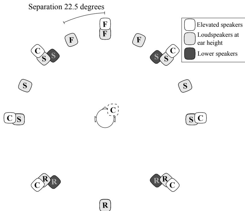
**Figure 4.18.** Reproduction setup with 24 speakers at three heights, the late reverberation of the IRs is distributed to speaker groups **Front (F)**, **Side (S)**, **Ceiling (C)**, **Rear (R)**.
