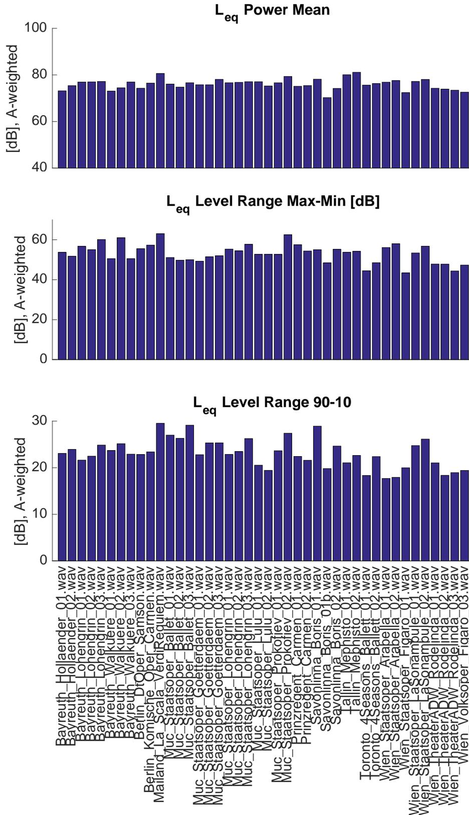
Figure 6.11. A-weighted sound pressure level and level ranges, Opera performances.
