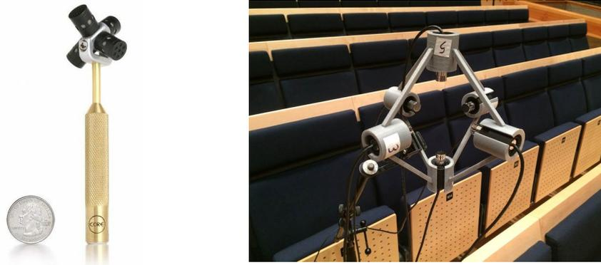
**Figure 2.9.** Arrays for directional measurements: TetraMic (left, photo from Core-Sound) and 6-ch array (right) with 10 cm distance between capsules
