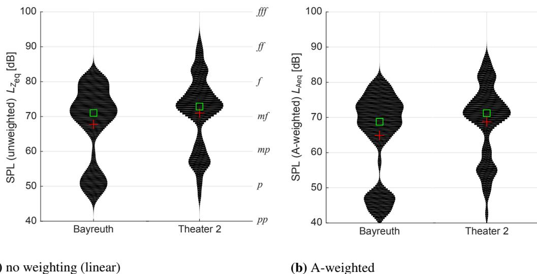
**Figure 6.7.** Comparison of level histograms without and with frequency weighting for a 59 seconds excerpt of Lohengrin.
