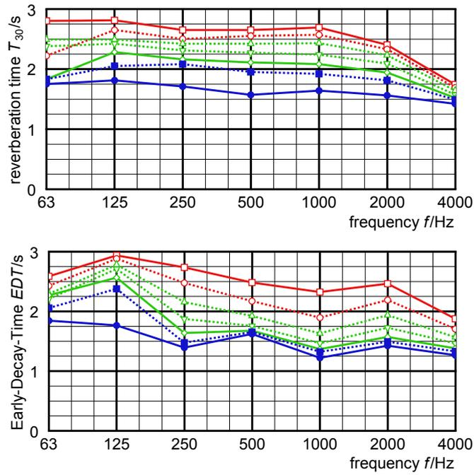
**Figure 3.5.** Measured reverberation time  $T_{30}$  (top) and early decay time EDT for the seven acoustic conditions, with and without electronic room acoustics system. Colors indicate the overall judgment in the listening test (green: “good, appropriate”).
