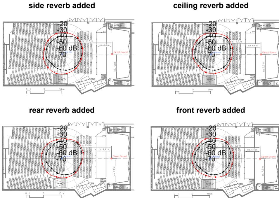
**Figure 4.15.** Ground view / lateral plane of Konzerthaus Detmold with the configurations for late reverberation (after 80 ms). Black denotes the natural late energy, the stimuli are shown in red with added reverberation.
