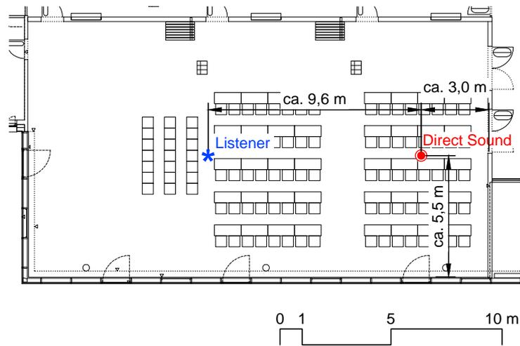
**Figure 2.2.** Plan of the lecture hall with a typical test arrangement.
