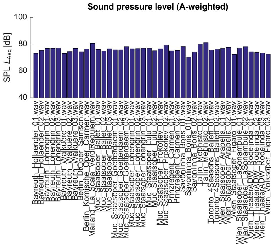
Figure 5.18. A-weighted sound pressure level and level ranges, Opera performances.
