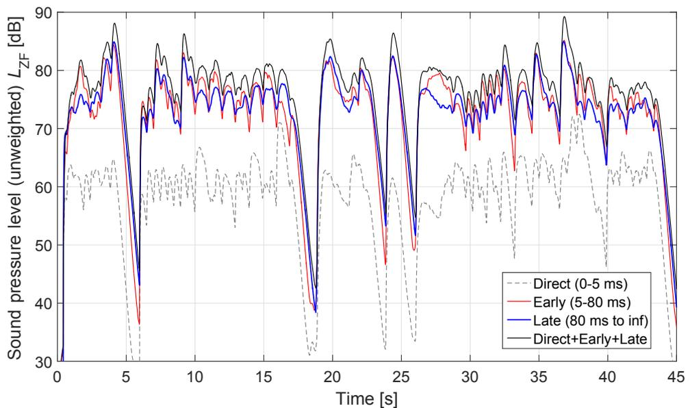
**Figure 5.6.** SPL over time for an Oboe playing in a simulated concert hall, convolved with the different time windows of the impulse response. “inf.” stands for infinity, i.e. end of the impulse response.
