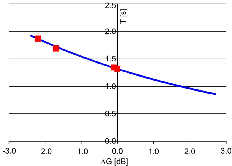
**Figure 3.19.** Relationship between change in strength and reverberation time for maintaining equal reverberance, calculated using Equation 3.4. Red points are data from Table 3.3.
