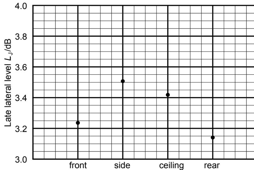
**Figure 4.16.** Late lateral level ( $L_J$ , 125-4000 Hz) for the modified directional sound fields, e.g. condition “front” with electronically added late reverberation from the front. Strength reference calculated from room volume and measured reverberation time.
