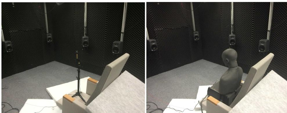
**Figure 4.31.** Measurement setup with increased backrest for array-(left) and dummy-head measurement (right).
