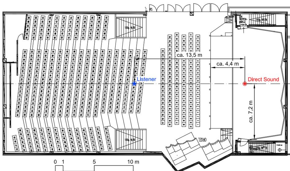
**Figure 4.11.** Konzerthaus Detmold with the receiver (left) and the direct sound loudspeaker on stage (right).
