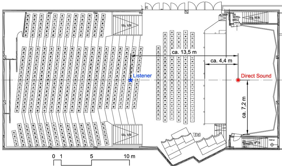
**Figure 2.5.** Plan of the Konzerthaus Detmold with a typical test arrangement.
