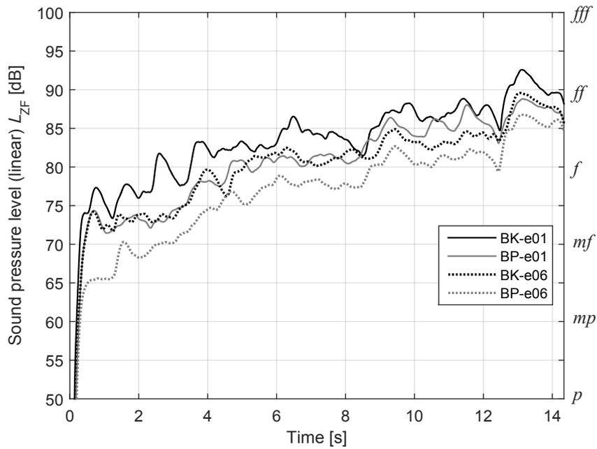
**Figure 5.23.** Linear sound pressure level over time for the four stimuli in original condition
