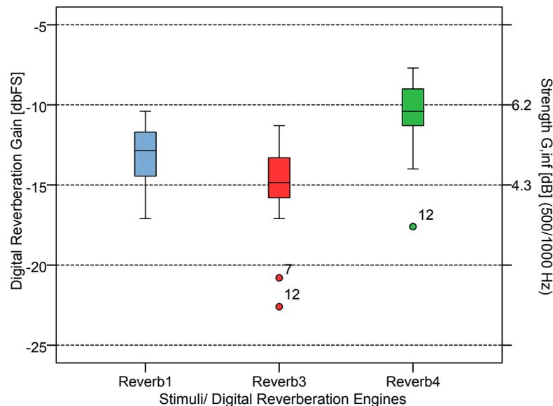
**Figure 3.17.** Boxplot with reverberation gains as set by 14 participants for *equal reverberance*. The median values were used for the measurements presented in table 3.3 and following.
