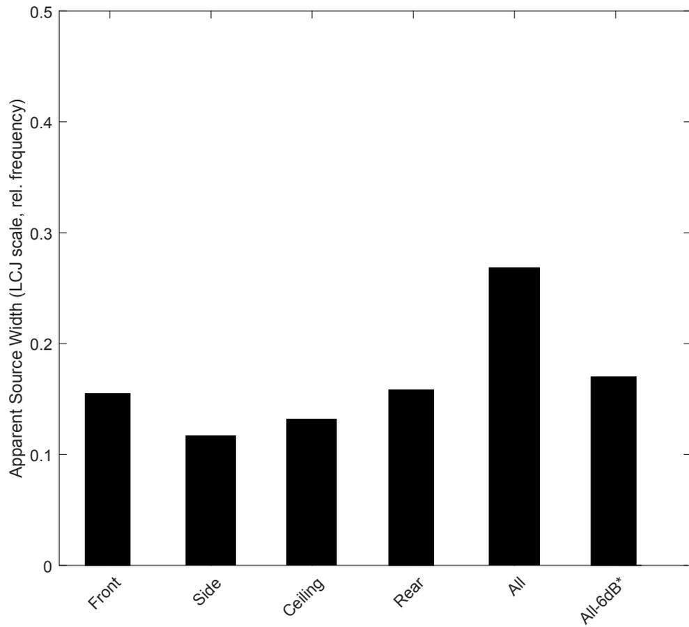
**Figure 6.4.** Apparent Source Width (ASW) for different directions of late energy.
