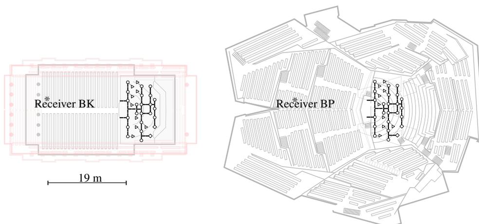
**Figure 4.17.** Groundplan of the Berlin Konzerthaus (left) and Philharmonie (right) with loudspeaker orchestra on stage.
