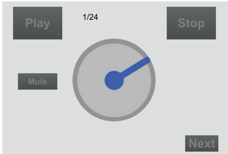
**Figure 4.22.** User interface for adjustment test (Exp. 2). The blue endless dial changes the level of the variable late reverb direction, 'mute' silences it.
