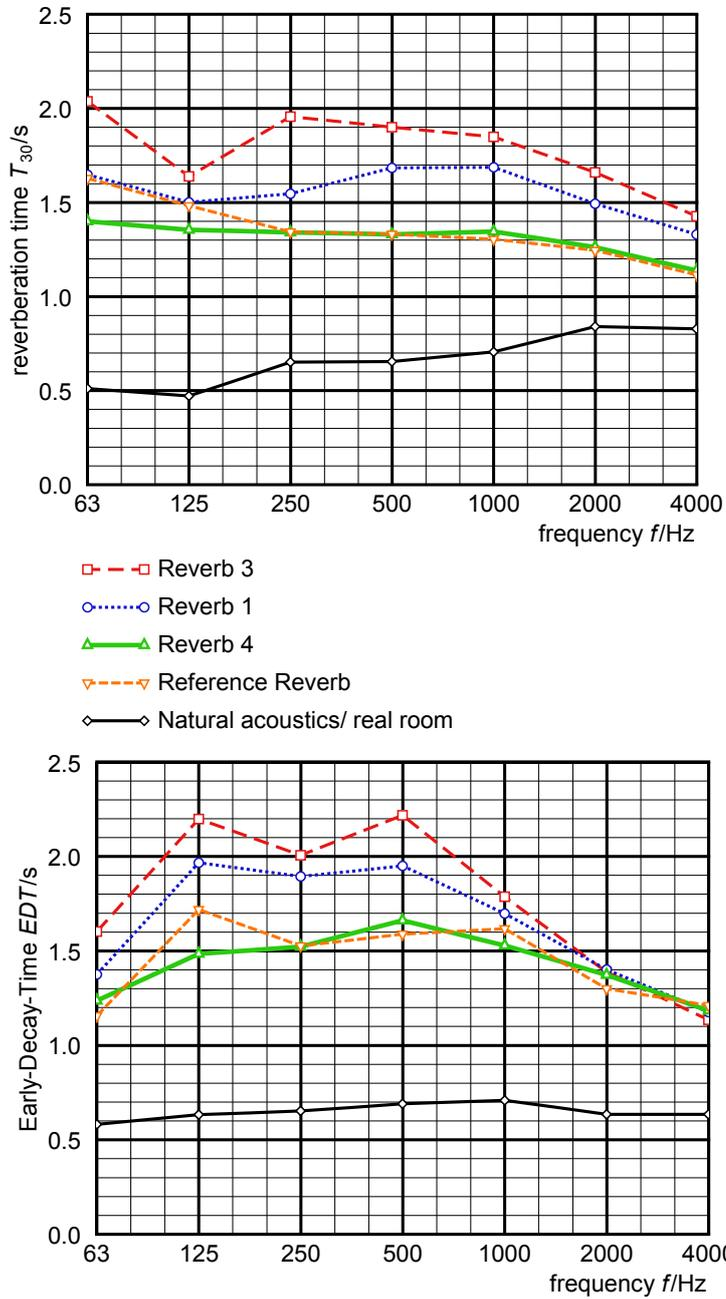
**Figure 3.18.** Reverberation time  $T_{30}$  (top) and early decay time EDT for the different acoustic situations as set by the participants for equal reverberance.
