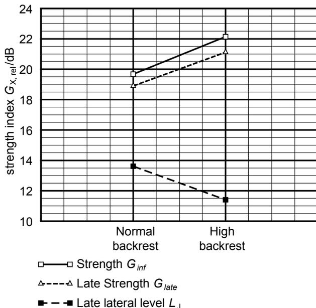
**Figure 4.29.** Strength indexes for the two chair versions in the synthesized diffuse sound field (Averaged 500/1000 Hz for  $G$  values and as well as for  $L_J$  for comparability). Virtual room, thus arbitrary gain/strength values.
