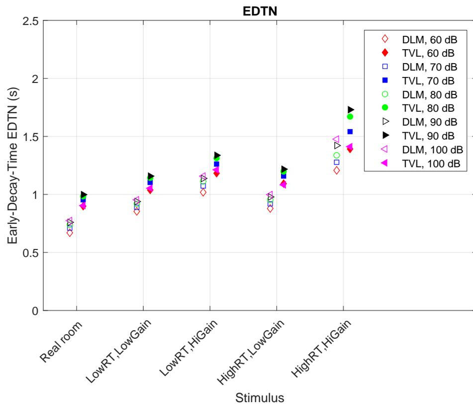
**Figure 3.24.** Loudness-based early decay time ( $EDT_N$ ) for Loudness models DLM (left) and TVL (right, filled) for different input levels for **Experiment 1 in Section 3.3**
