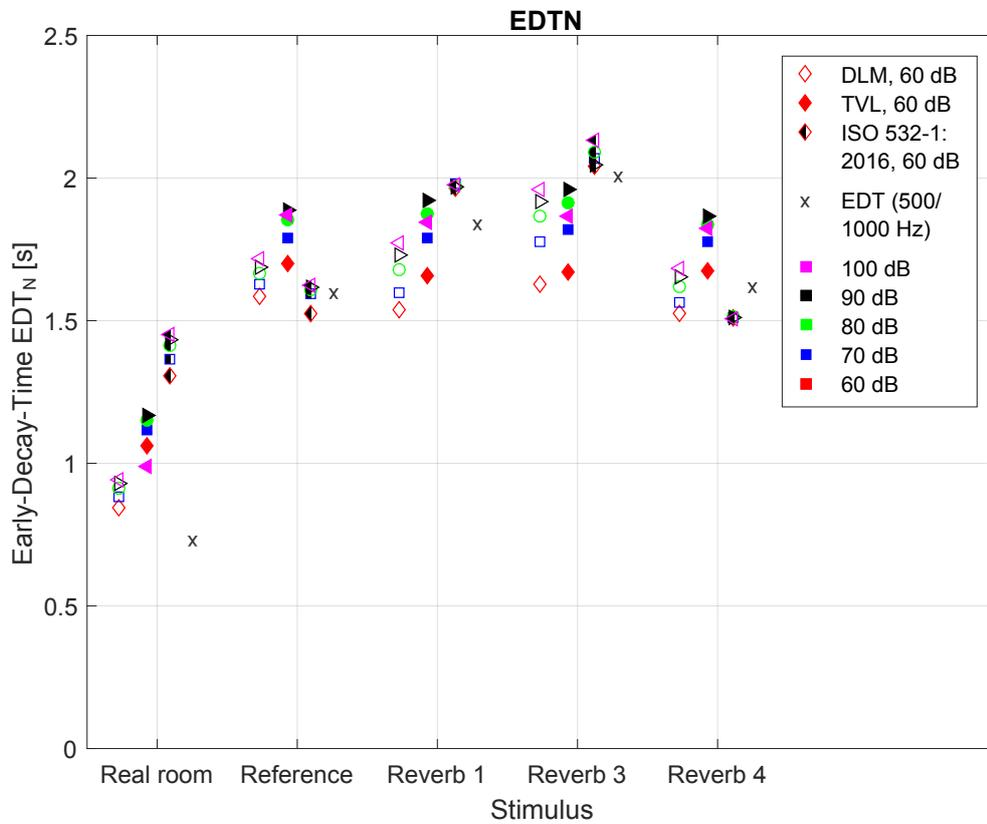
**Figure 3.23.** Loudness-based early decay time ( $EDT_N$ ) for Loudness models DLM (empty markers), TVL (filled), ISO532-1 (semi-filled) and regular EDT (x) for different input levels.
