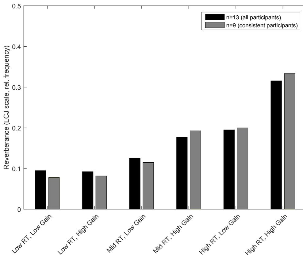
**Figure 3.15.** Perceived amount of reverberation for experiment 2 with all 13 listeners (consistency  $T > 0.4$ ) in black and more consistent 9 listeners ( $T > 0.6$ ) in grey.
