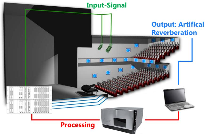
**Figure 1.4.** Schematic for room enhancement system *Vivace*, Figure adapted with permission from Müller-BBM ASO.
