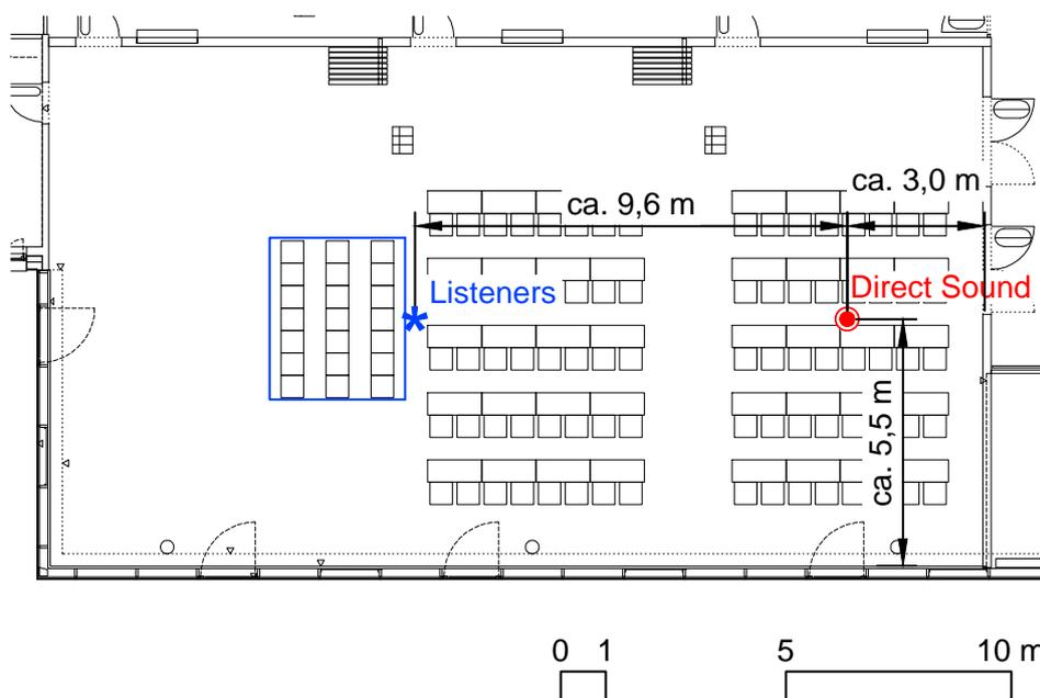
**Figure 3.9.** Ground view of the lecture hall with the test arrangement. Listeners were seated in the area marked in blue.
