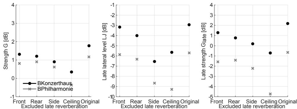
**Figure 4.21.** Parameters for the different conditions, Avg. 500/1000 Hz for  $G$  and 125-1000 Hz for  $L_J$ ,  $G_{\text{late}}$  (Exp. 1).
