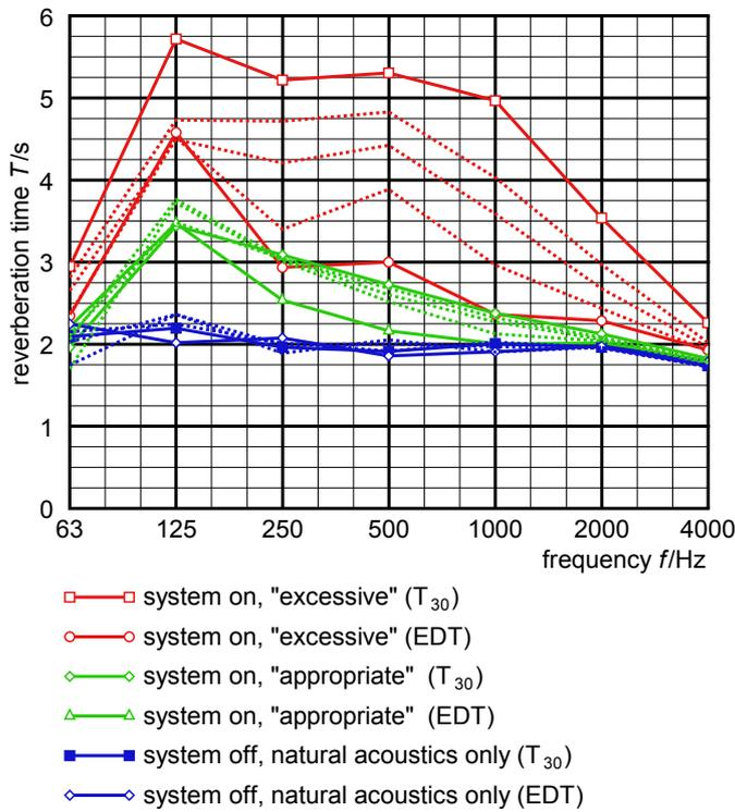
Figure 3.29. Reverberation times for different evaluation ranges in an opera venue with enhancement system. EDT and  $T_{30}$  are labeled and in solid lines, dotted in between are  $T_{10}$ ,  $T_{15}$  and  $T_{20}$ .
