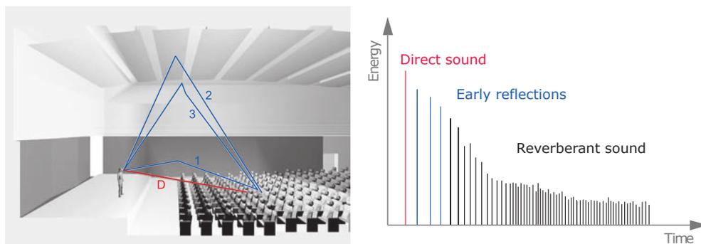
**Figure 1.1.** Schematic representation of sound built-up, Figure from [7, p. 12]
