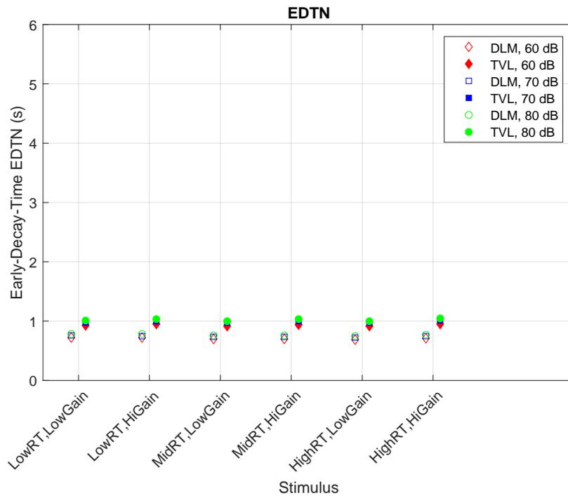
**Figure 6.1.** Loudness-based early decay time ( $EDT_N$ ) for Loudness models DLM (left) and TVL (right, filled) for different input levels **Experiment 2**
