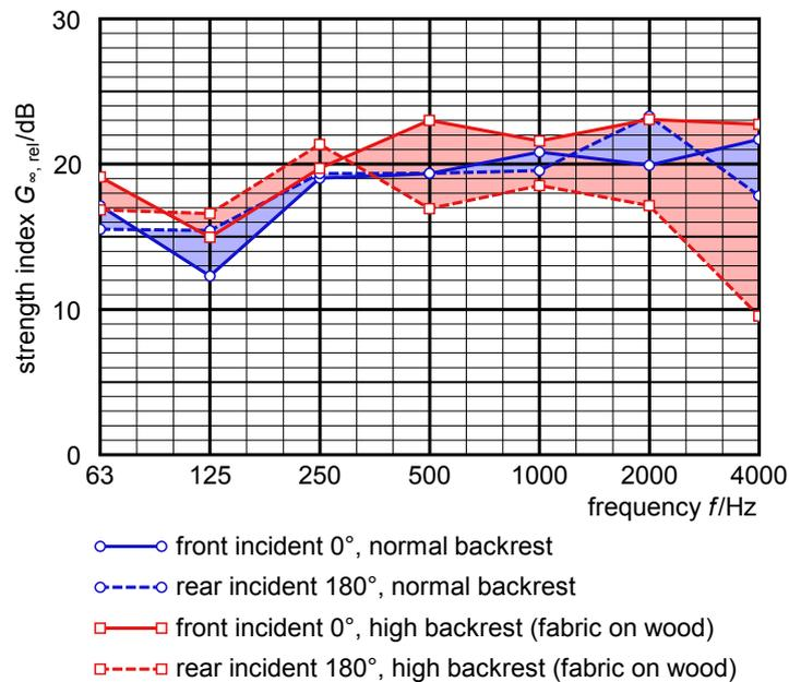
**Figure 4.28.** Strength  $G$  measured with the two chair versions and frontal and rear sound (binaural measurement, results from left ear only). Virtual room, thus arbitrary gain/strength values.
