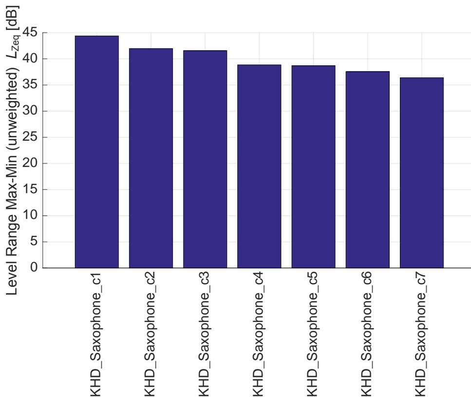
Figure 5.4. Increasing reverberation (c1 to c7) reduces the dynamic range of a lively saxophone signal.
