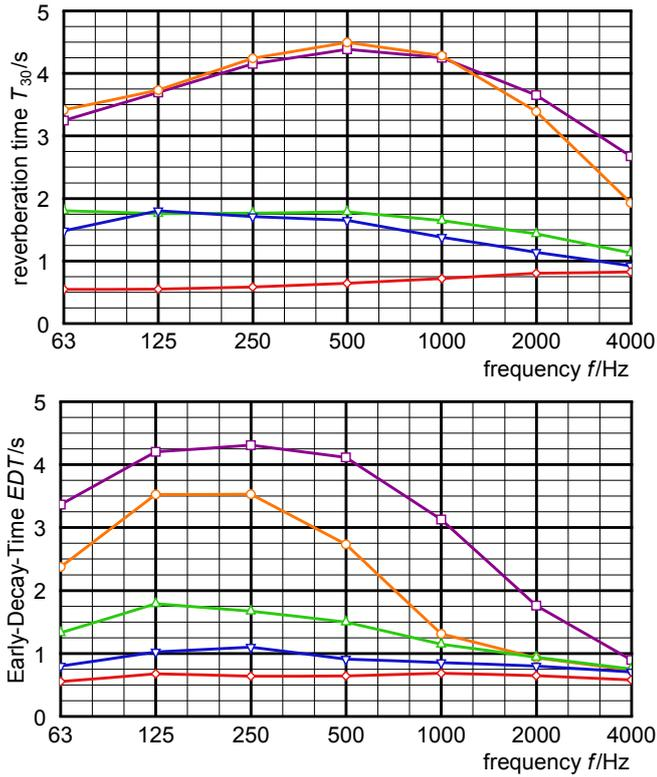
**Figure 3.10.** Reverberation time  $T_{30}$  (above) and early decay time EDT (below) for the five conditions (Experiment 1).
