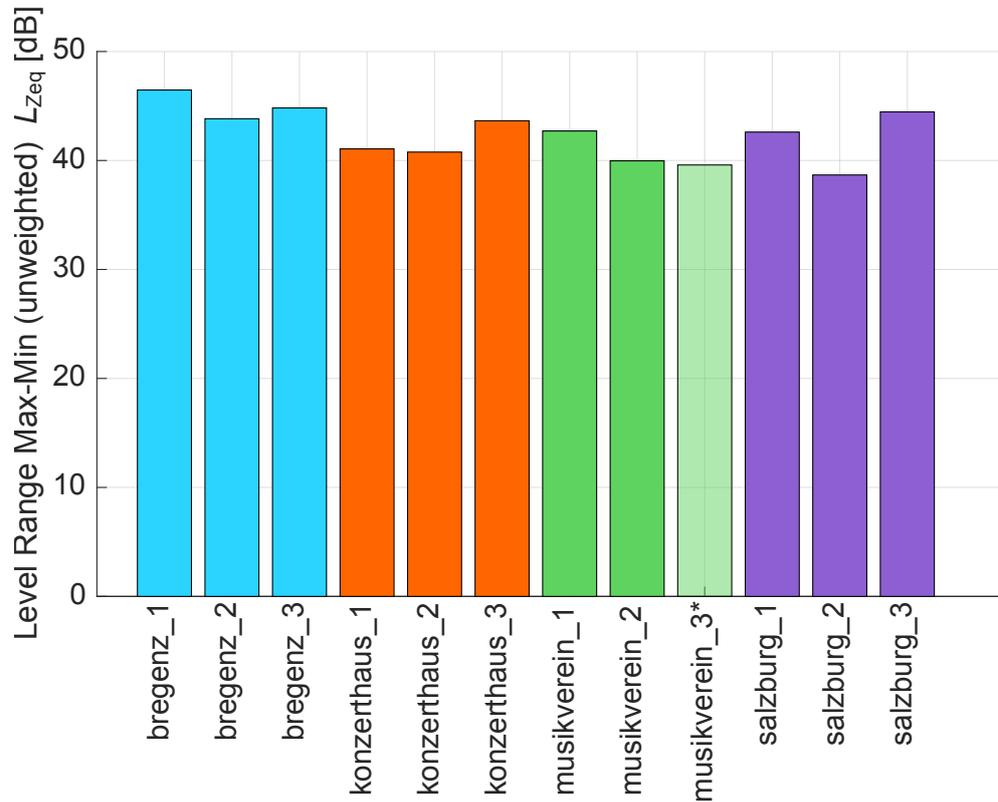
**Figure 5.9.** Level range for a 67 second Bruckner excerpt, recorded in four halls at each three comparable receivers positions.
