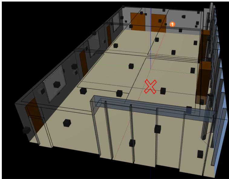
**Figure 2.3.** 3D-model view of the lecture hall. Black rectangles represent enhancement loudspeakers. The orange circle (1) shows the position of the direct sound speaker for a test, “X” of the listener.
