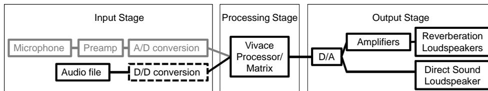
**Figure 2.1.** Flow chart with the working principle of an enhancement system as used in the thesis (black).
