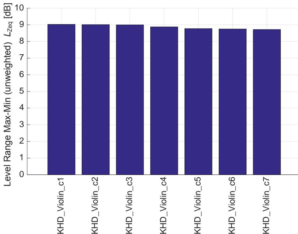
Figure 5.5. Increasing reverberation (c1 to c7) reduces the dynamic range of the Violin signal, but less so as the signal is not changing as much over time.
