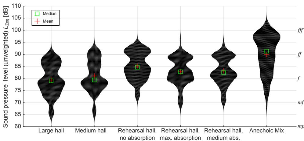
**Figure 5.16.** Level histograms for the five convolved signals and the anechoic source material.
