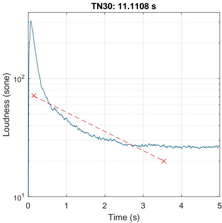
Figure 3.26. Plot of the loudness decay with regression for Reverberation Time ( $T_{N30}$ ) for Loudness model TVL at level 100 dB (Experiment 2 in Section 3.3, stimulus “HighRt, LowGain”).
