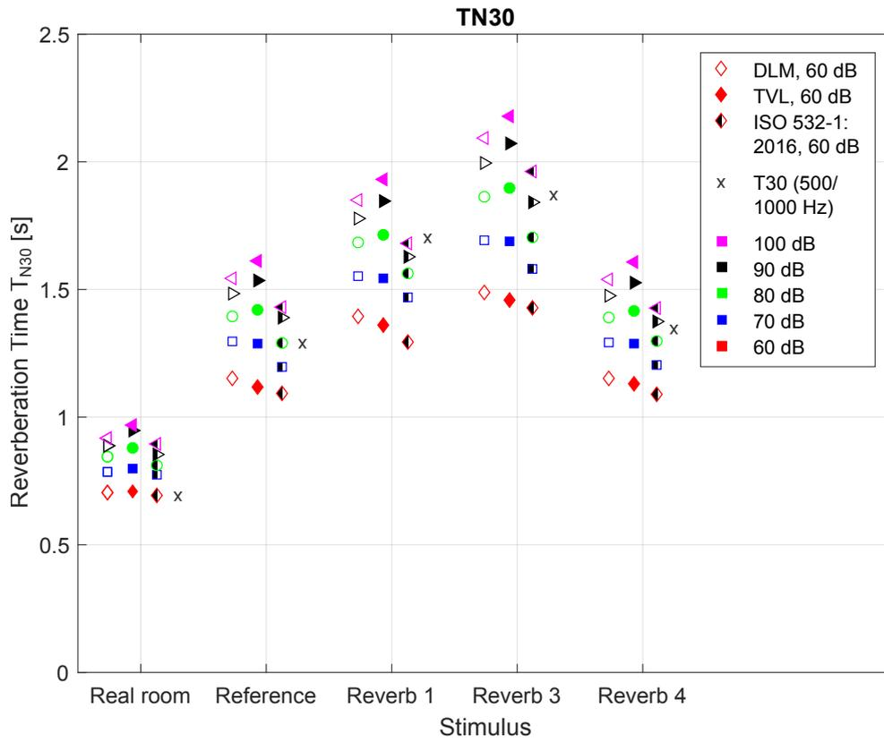
**Figure 3.22.** Loudness-based Reverberation Time ( $T_{N30}$ ) for Loudness models DLM (empty markers), TVL (filled), ISO532-1 (semi-filled) and regular  $T_{30}$  (x) for different input levels.
