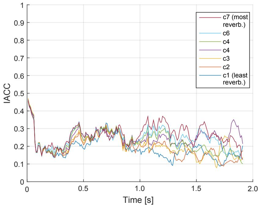
**Figure 4.9.** IACC over time, unfiltered, for increasing amount of reverberation (“c1” with least reverberation to “c7” with most) in Konzerthaus Detmold, energy before 80 ms stays constant (setup see Section 3.2).
