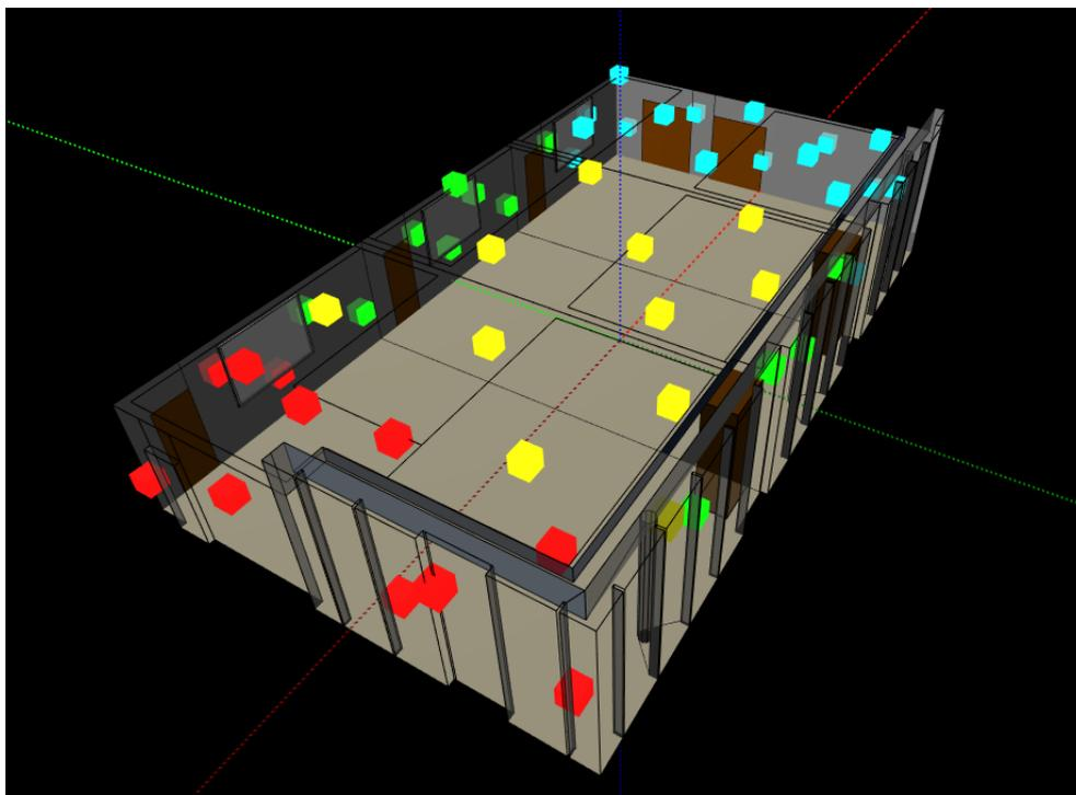
**Figure 4.3.** 3D-Model Lecture Hall with loudspeakers and directional late energy groups (colored): “front” speakers (blue), “rear” speakers (red), “side” speakers (green) and “ceiling” speakers (yellow).
