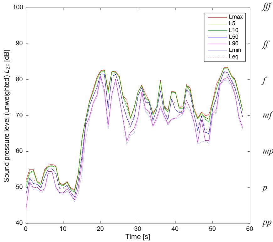
**Figure 5.2.** SPL over time, different percentile levels for a 59 sec excerpt of “Lohengrin” with a brief quiet section and a longer mezzoforte-forte part. Dynamic notations suggested to be appropriate for an orchestra as a whole.
