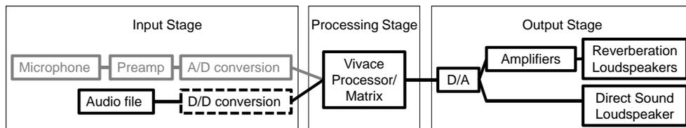
**Figure 2.1.** Flow chart with the working principle of an enhancement system as used in the thesis (black).
