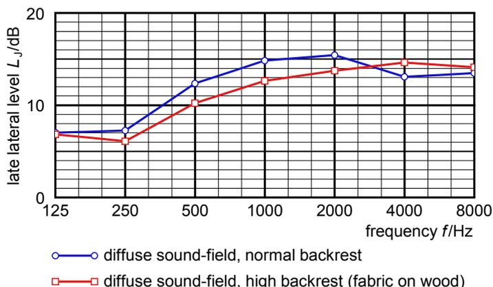
**Figure 4.30.** Late lateral Level  $L_J$  for the two chair versions in the synthesized diffuse sound field. Virtual room, thus arbitrary gain/strength values.
