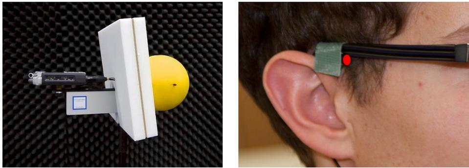
**Figure 2.8.** Pseudo-Dummy head (left) and location of miniature microphone on human listener (right): The microphone is marked with red, no tape was attached for the actual recordings.
