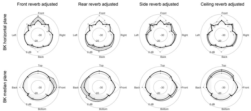
**Figure 4.25.** Spatial plots for Berlin Konzerthaus. Late energy (80 ms - inf) for the original situation in solid black, participants' median adjustments are shaded grey. Dotted grey lines show early energy (0-80 ms).
