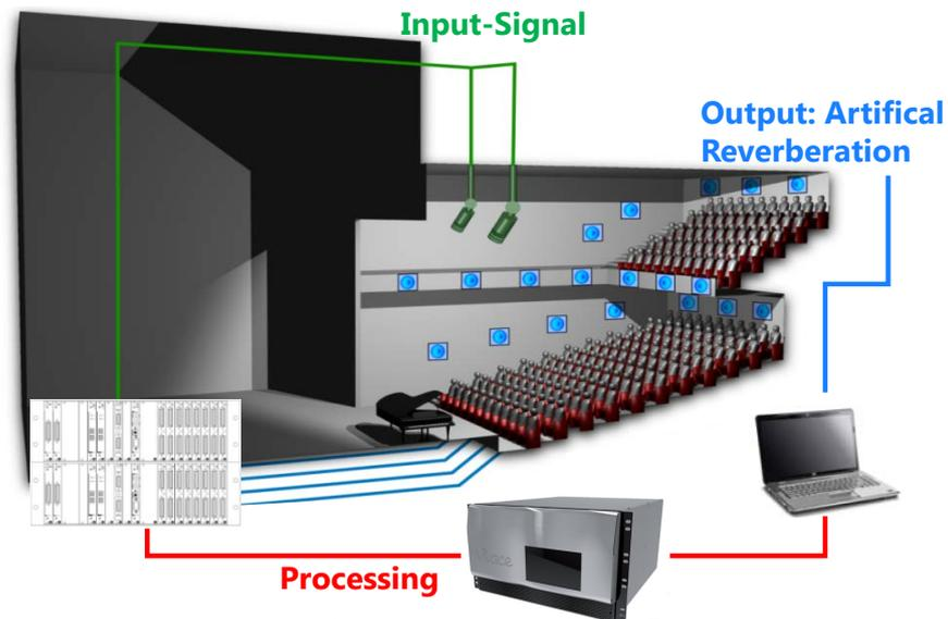
**Figure 1.4.** Schematic for room enhancement system *Vivace*, Figure adapted with permission from Müller-BBM ASO.
