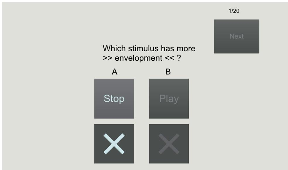
**Figure 2.10.** Graphical user interface for a paired comparison test: Envelopment, i.e. being surrounded by sound, has to be judged between the stimuli A and B.
