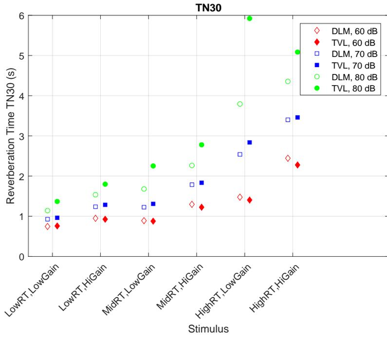
**Figure 6.2.** Loudness-based Reverberation Time ( $T_{N30}$ ) for Loudness models DLM (left) and TVL (right, filled) for different input levels **Experiment 2**
