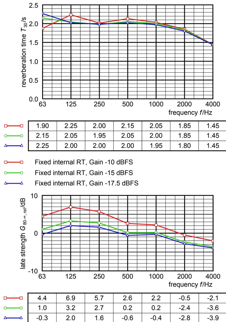
**Figure 3.27.** Measured reverberation times (top) and -levels (bottom) in Konzerthaus Detmold for different gains of the enhancement system set to the same internal decay time.
