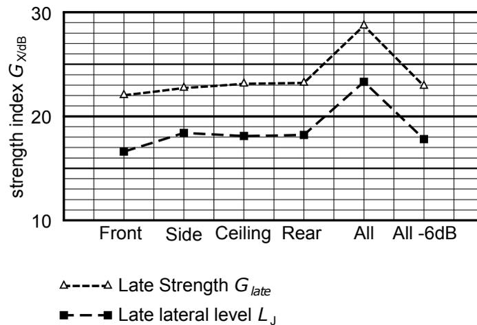
**Figure 4.8.** Late sound strength and late lateral level for the different late energy directions. Strength reference calculated from room volume and measured reverberation time.
