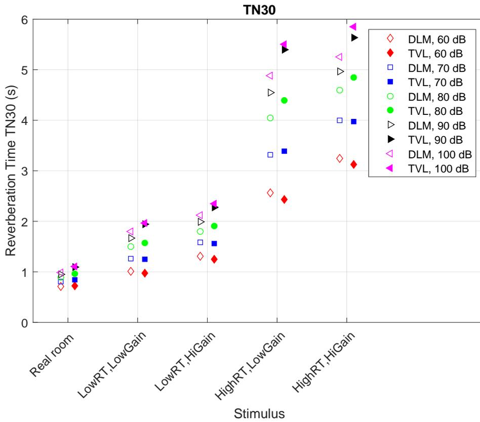
Figure 3.25. Loudness-based Reverberation Time ( $T_{N30}$ ) for Loudness models DLM (left) and TVL (right, filled) for different input levels Experiment 1 in Section 3.3
