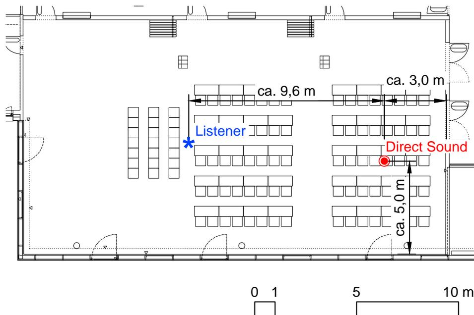
**Figure 3.16.** Ground plan of the lecture hall with the test setup.
