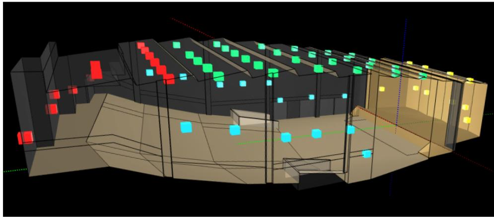
**Figure 2.7.** 3D-model view of the Konzerthaus Detmold. Rectangles in different colors represent loudspeaker channels used for the artificial enhancement.
