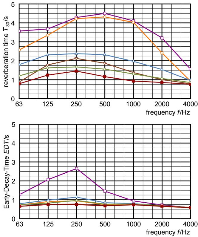
**Figure 3.13.** Reverberation time  $T_{30}$  (top) and early decay time EDT for the six conditions (Experiment 2).
