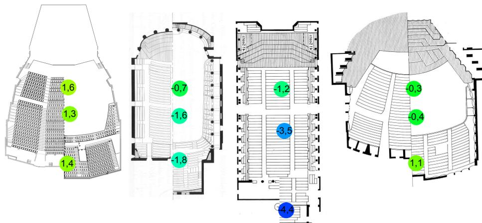
**Figure 5.8.** Groundplans and receiver positions of the four halls with each receivers 1, 2 and 3 from stage to the back of the hall. Data from the author [43], plans from Müller-BBM and literature [19]. For reference, clarity  $C_{80}$ , the energy ratio between late and early energy is shown.
