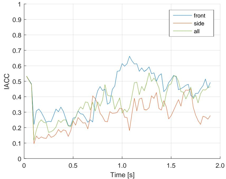
**Figure 4.7.** IACC over time calculated in 25 ms windows, unfiltered. Artificial late reverberation was added from the front speakers (blue), all speakers (green) and side speakers (red).
