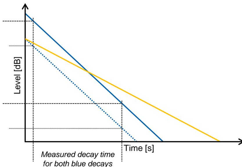
**Figure 3.1.** Schematic representation of two decays with the same (relative) decay time but different reverberation levels (solid and dotted blue line). Also, a longer, quieter decay (yellow) might evoke the same reverberance as a louder, but shorter decay (solid blue).
