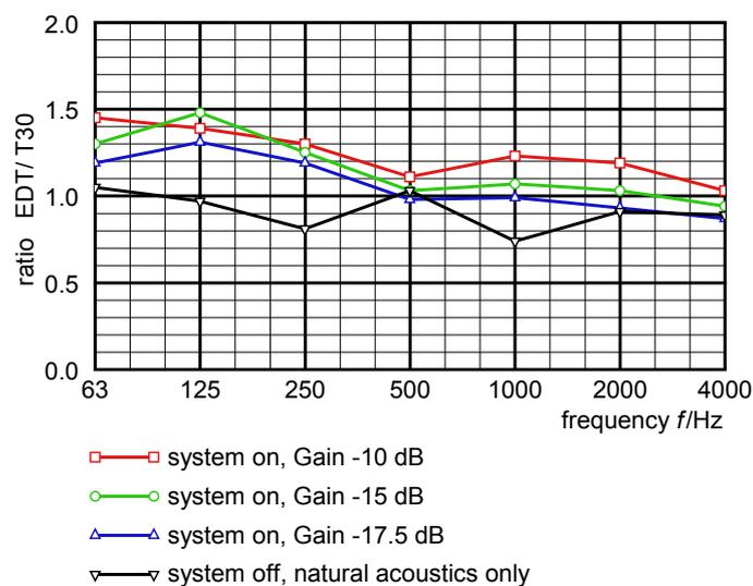
**Figure 3.28.** Ratio of EDT to  $T_{30}$  for the setup in Konzerthaus Detmold.
