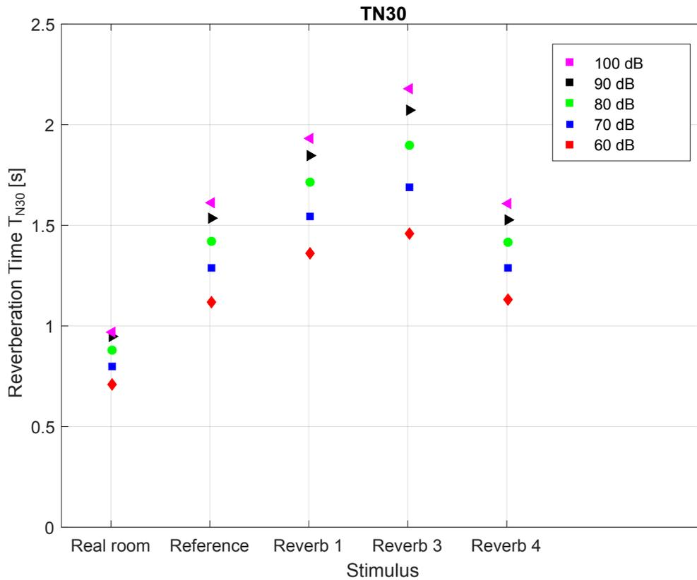
**Figure 3.21.** Loudness-based Reverberation Time ( $T_{N30}$ ) for different input levels in the reverberance matching experiment.
