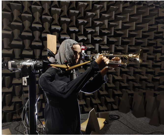
Figure 1.5: A high resolution directivity measurement setup of a trumpet with mannequin, employing a 3D turn table, and offering a 5^\circ spatial resolution resulting 2,522 unique measurement points (from [67]).
