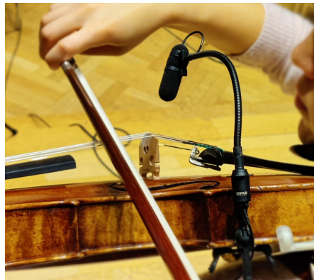
Figure 2.2: Position and orientation of DPA clip-on microphone on violin.
